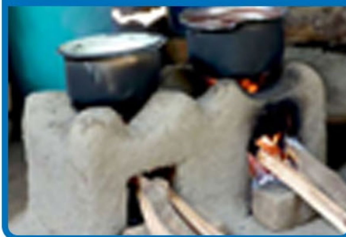
Chitetezo Mbaula biomass stove (ICS). Combustion chamber is insulated.
